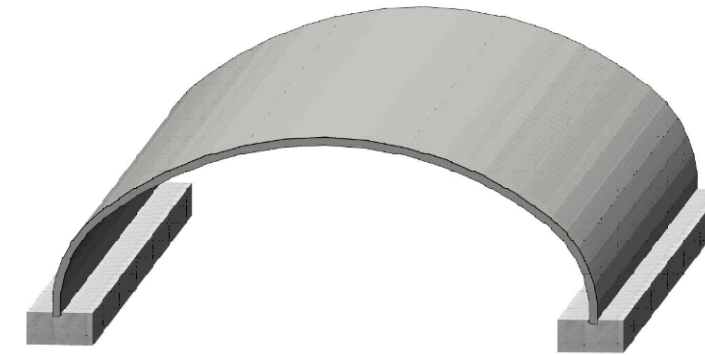
PROPOSED OPEN-BOTTOM ARCH CULVERT - ISOMETRIC VIEW NOT TO SCALE
